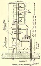
Fig. 234.—Remote mechanical oil circuit-breaker arranged in masonry structure.\*
